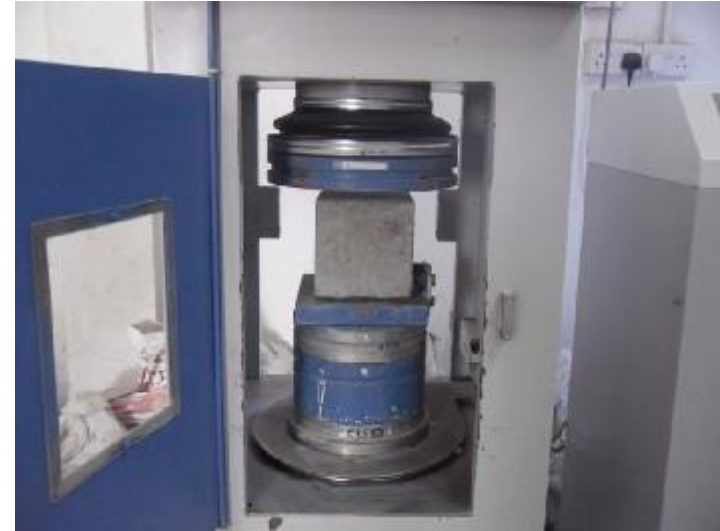
Compressive strength (SAI) testing of cement block
