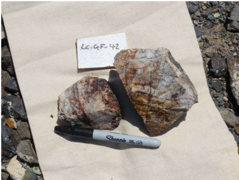
Example of epithermal quartz vein material sampled from the Power Line zone. This sample assayed at 18.3 g/t Au, 43.6 g/t Ag and 11,300 ppm Pb
