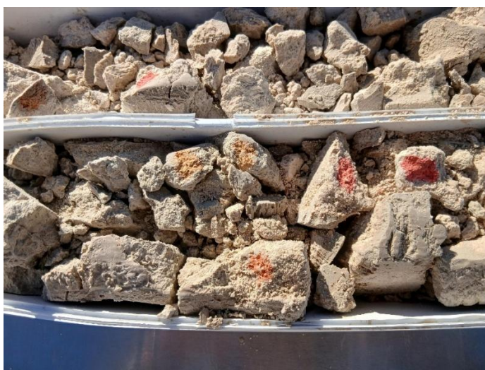
Above. Core samples of sepiolite clay. Orange red spots result from chemical field tests using a chemical stain to make an initial positive identification of magnesium bearing sepiolite clay.
