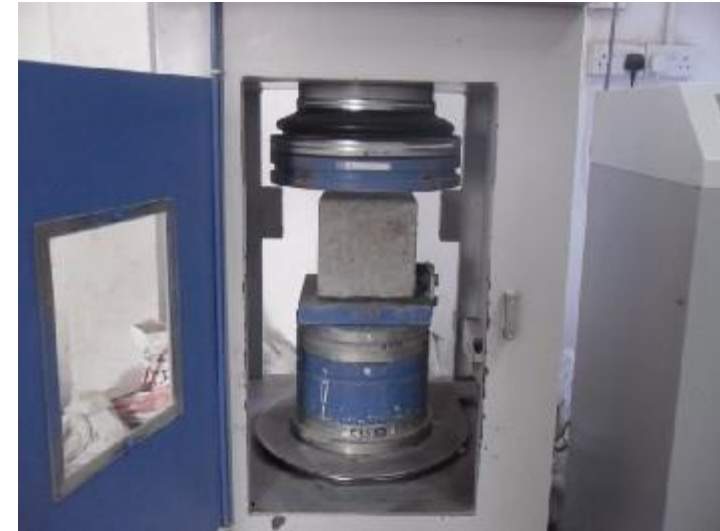
Compressive strength (SAI) testing of cement block
